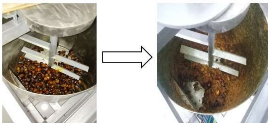
Figure 3. The test of FFB digester machine
